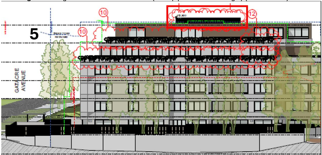
Figure 4: Lodged s4.55 southern elevation (rooftop plant 1.29m in height) (Source: PBD)
