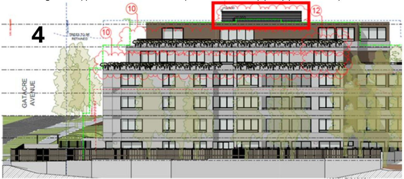
Figure 4: Lodged s4.55 southern elevation (rooftop plant 1.29m in height) (Source: PBD)
